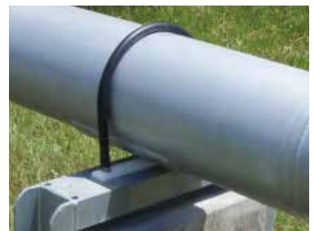
I-Rod® eliminates the crevice by minimising the contact area and allowing any moisture to evaporate. It's also much easier to inspect.
